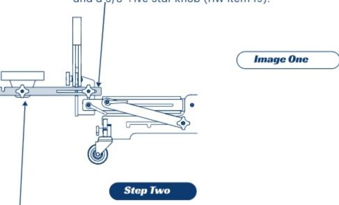
Place the Tool Tray (PW item 8) in between the two Small Rails (PW item 9) and attach them through the 3/8" slots of the Small Rails with the 3/8" x 2 1/4" Carriage Bolt (HW item 17) along with a 3/8" Flat Washer (HW item 18) and a 3/8" Five Star Knob (HW item 19). The Tray is able to slide back and
