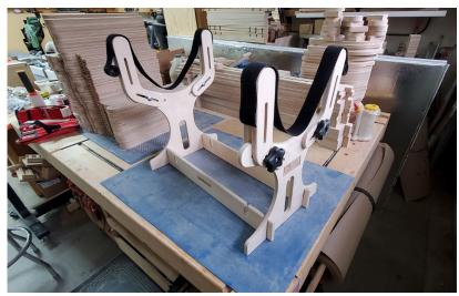
I give you about 6 feet of Velcro One-Wrap for the straps, cut it at about 60% to 40% to make two straps. Straps just lay over Velcro arms and adjust accordingly.
