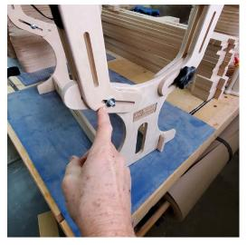
Knobs go on the outside with 5/16" washers first. Adjust arms to about ½" to 1" from fuselage to minimize swaying.
