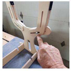
Install the 5/16" lag bolt from the inside of the stand into the slot. This will give you plenty of flexibility. You can also reverse the arms for narrow fuselages.
