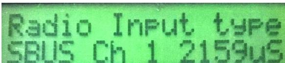
If Futaba SBUS is used, it displays the channel it is using (CH1 on the picture) and the current value read on this channel.
