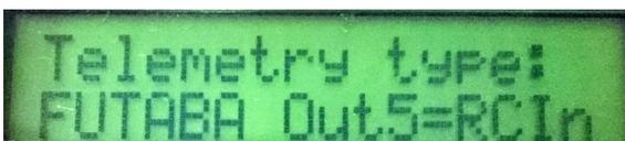
Using the SBUS to receive the gear command allows to free an receiver output for other use, and to free the RCIN input on the sequencer, in this case this connector reconfigures as an output for the 5<sup>th</sup> output of the sequencer.
