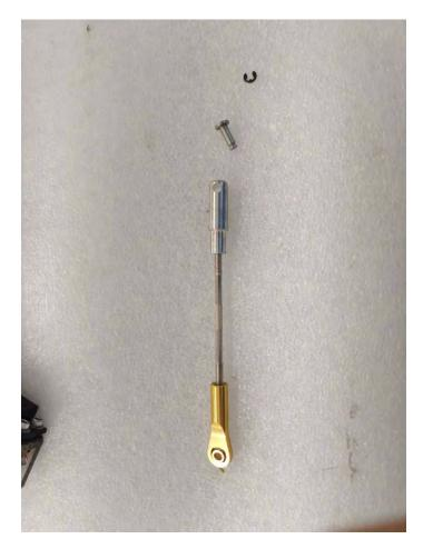
推杆安装 Push rod installation
