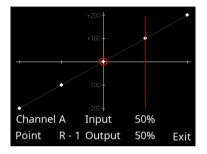
The procedure is very simple: use buttons I and II to select the point on the curve which you wish to change, then press the SET button. The servo automatically moves slowly to the corresponding point. Now you can alter the servo curve at this point using buttons I and II.
