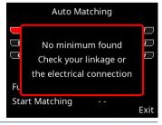
A matching process for three servos takes about 30 - 40 seconds. You can follow the current consumption directly on the screen. When the matching is finished, use the transmitter stick to run the servos to all five points. A quiet buzz from the servos in one or other position is normal. If the buzzing stops when you touch the control surface lightly with your finger, then this shows that the matching process has worked accurately.
