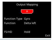
Press the SET button to select the output. On the next screen you can now define the output:
