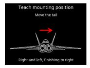
This is accomplished by moving the model in the directions shown in the graphic display: first move the tail of the model up and down two or three times. You will see that the elevators follow this movement every time - the direction of effect is not important at this stage.
