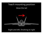
The orientation of the gyro is established by moving the model in the directions shown on the screen: to ensure that detection is absolutely reliable, move the tail of the model smoothly up and down several times before holding the tail up until the elevators return to neutral. The direction of effect is not important at this stage. The diagram of the little afterburners on the screen lets you know whether the movement was sufficient!
