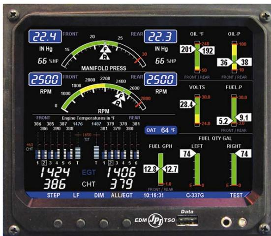
Twin Center line thrust Configuration
