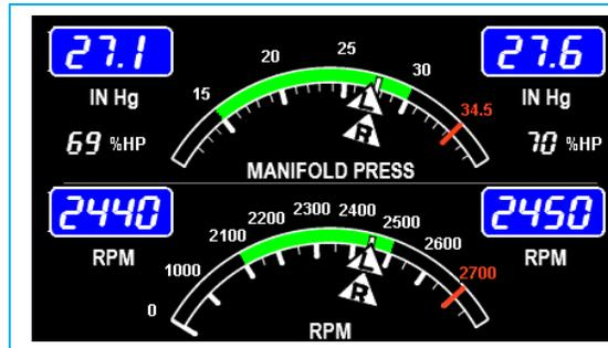
Percent horsepower is displayed digitally below each MAP digital readout.
